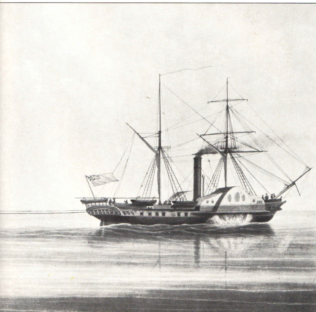
The Alecto , paddle-wheels thrashing the sea, hauls at the screw-vessel Rattler during a test of strength between propeller and paddle in 1845. The Rattler won easily.
