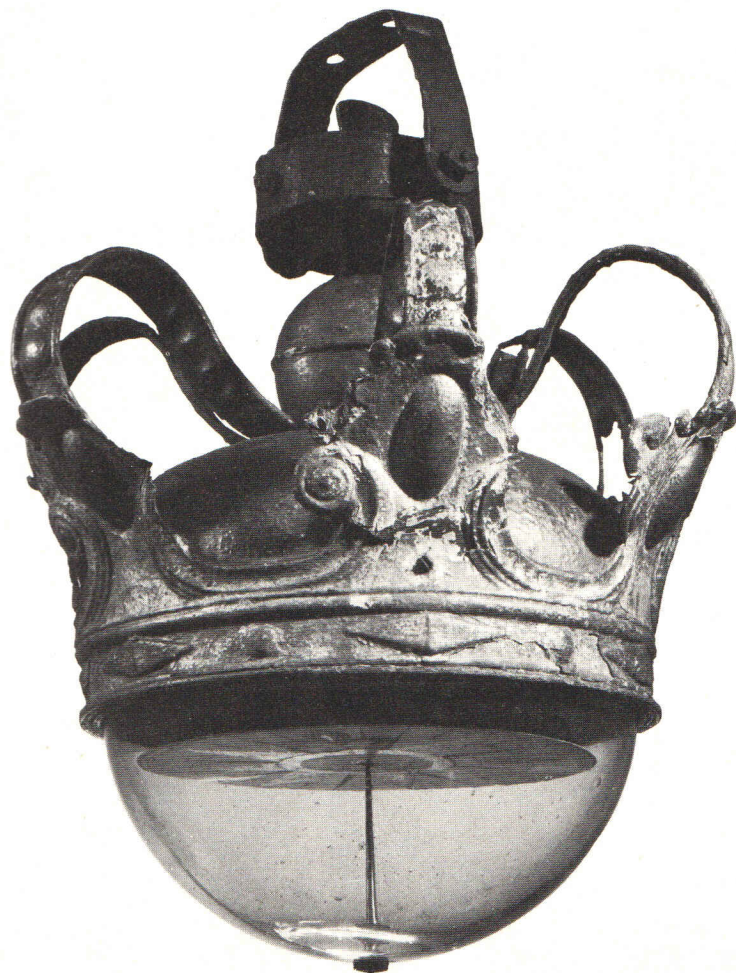
This crown-shaped hanging compass of 1790 was fixed to the ceiling of a captain's cabin so he could glance at it when working or lying down.
